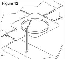
The optional hole saving brackets are installed and the speaker wire is attached to the bracket.
